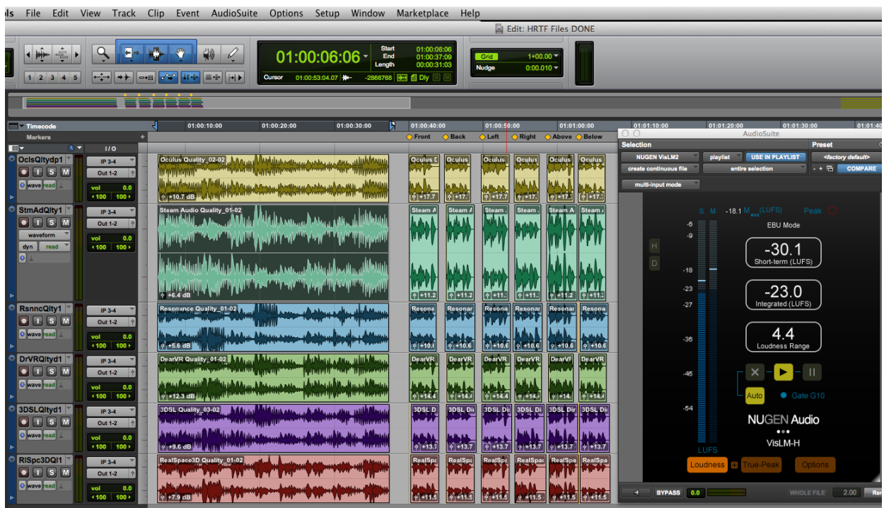
Figure 35: Audio files and loudness calibration as recommended in the EBU R128 standard.
