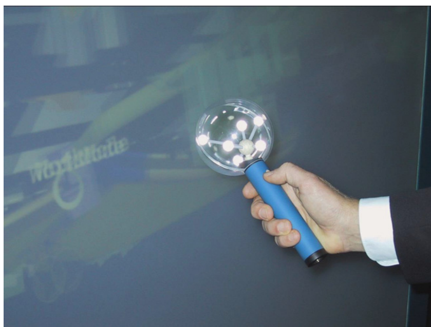
Fig. 6. An optically tracked wireless device with 6 DOF.
