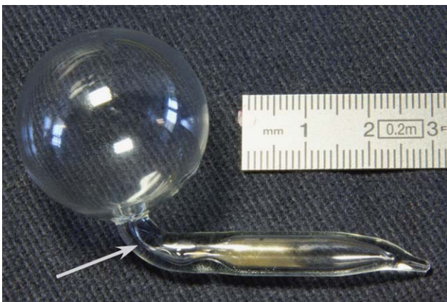
Fig. 1 Paraffin-coated Cs vapor cell. The small amount of the solid alkali metal is well visible in the sidearm. The arrow points to the capillary which reduces depolarizing collisions of vapor atoms from the cell with the solid Cs
