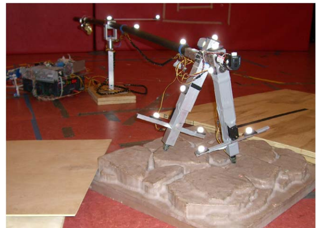
Fig. 10 Rough terrain experiment with the motion capture system. 12 markers are attached in the boom and legs
