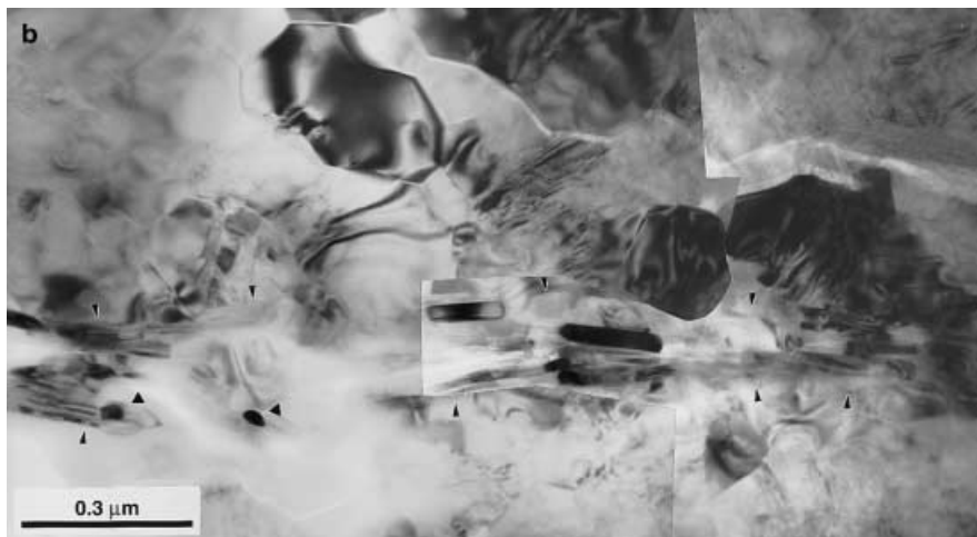
Fig. 5 a TEM image of ordered “as-is” (An54) labradorite deformed at 750°C, 1.5 GPa to \gamma=4.5 showing recrystallized plagioclase grains in the matrix of the sheared sample. The grains with high dislocation densities are portions of the old grains, and the dislocation-free grains are new grains that have more albitic (An34–36) composition than the starting material. b TEM image of a shear band in ordered (An54) labradorite (extending horizontally between the arrowheads), consisting of zoisite ( dark laths ) and albitic plagioclase ( small grains next to triangles ). Most of the grains within the shear band are dislocation-free, and zoisite grains are well aligned with the shear band boundaries. Recrystallized matrix plagioclase is observed above and below the shear band; note the coarser grain size
