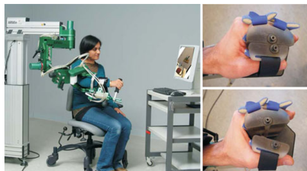
Fig. 1 ARMin III with a subject performing virtual ADL tasks ( left ) and the hand module ( right )
