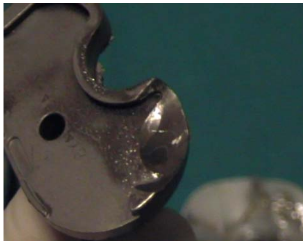
Fig. 5 Photograph showing retrieved tibial component showing an import usure on the medial side
