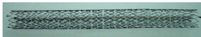
Figure 1 The Flype stent. Detail of the unconstrained stent showing strut design and tantalum radio-opaque markers.
