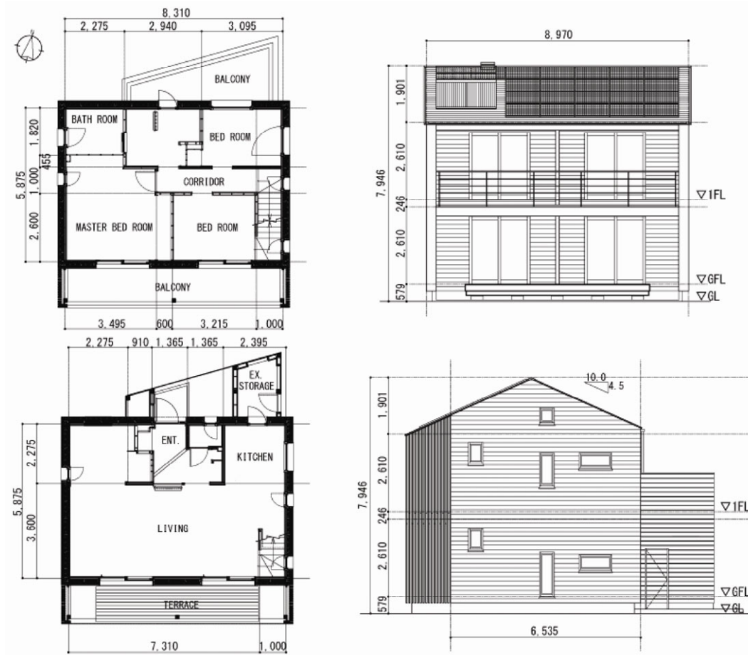
Fig. 6 Test House (in meters. upper left: floor plan of the 1st floor; lower left: floor plan of the ground floor; upper right: south facade; lower right: east facade)
