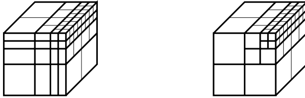
Fig. 5. Auxiliary shape-regular edge mesh \tilde{\mathcal{T}}_e (left) obtained from a macro-mesh \tilde{\mathcal{T}}_{e,m} (right)
