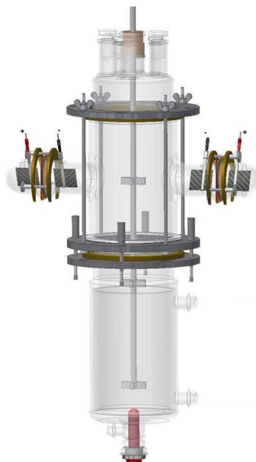
Fig. 5 3.2 L bioreactor with a microbial fuel-cell-like activity sensor. A cathode with a 0.5 M \text{K}_3\text{Fe}(\text{CN})_6 solution is positioned on the right, and the anode in the bioreactor solution is adjacent to it and separated from it by a Nafion proton exchange membrane
