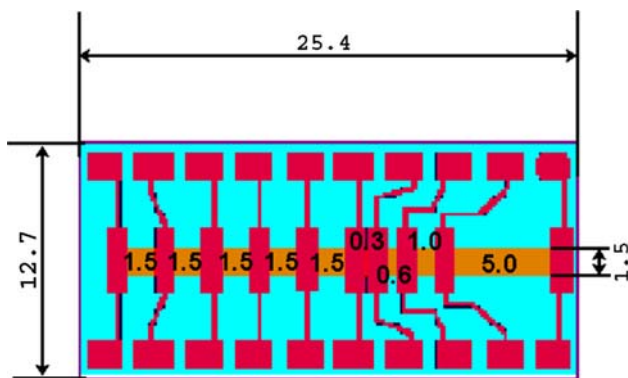
Fig. 1 Layout of the test sample for measurement of electrical properties
