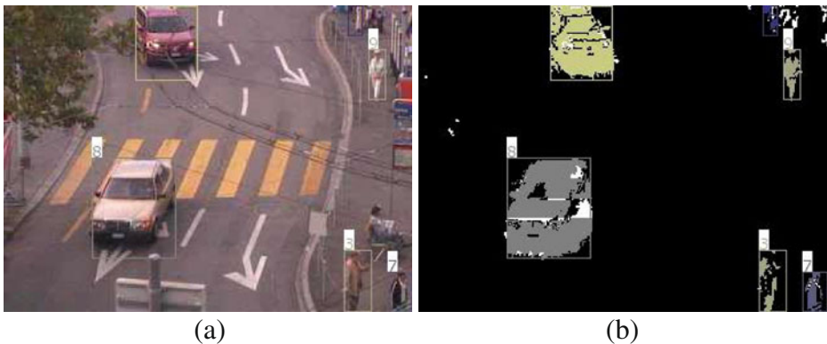
Fig. 6 Segmentation from the Central square sequence. The different size of the bounding box visualizes the different object classes. Unique object IDs are shown in the top left corner. Black pixels = background, white pixels = unassigned pixels \mathcal{N} , colored pixels = individual objects. a Camera view. b Segmentation
