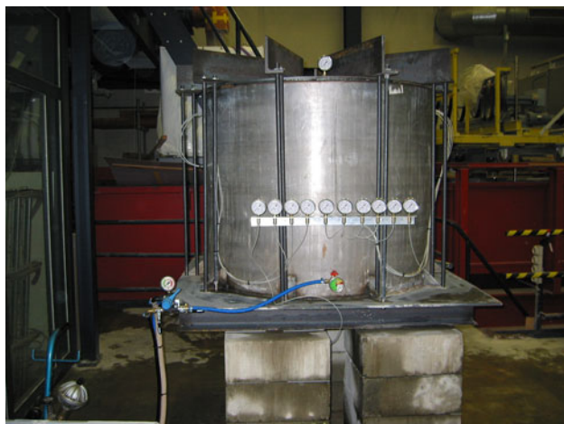
Fig. 7 View of the experimental set-up showing the vertical, cylindrical steel pressure vessel, the pre-stressed steel bars for stabilizing the bottom and top cap of the cylinder, the pressure gauges of the piezometers and the pump producing the external pressure (bottom left)
