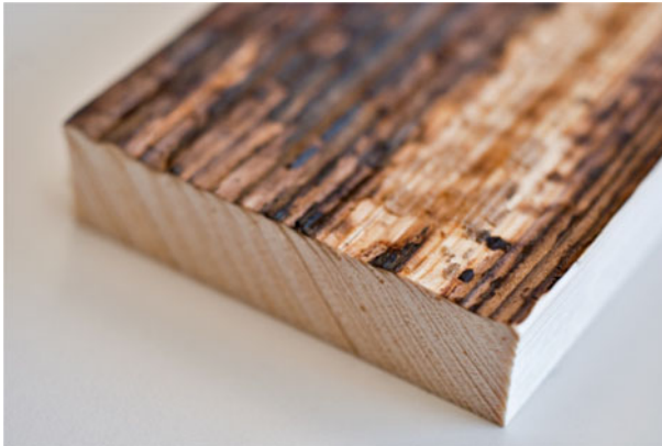
Fig. 4 Failure of welded wood specimens
