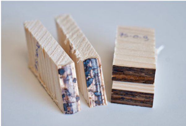
Fig. 3 Failure of off-axis samples: ( left ) rejected and ( right ) not rejected
