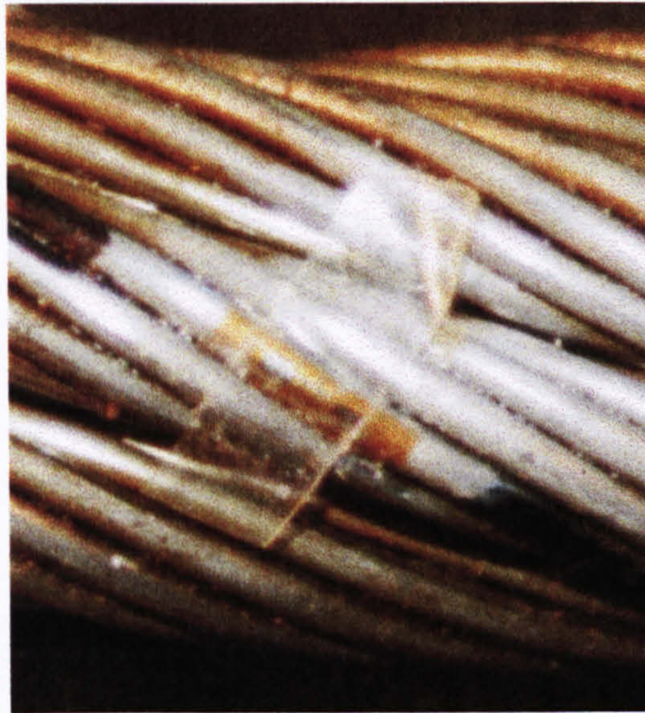
Figure 2.7. Enlarged picture of a strain gauge on a rope.
