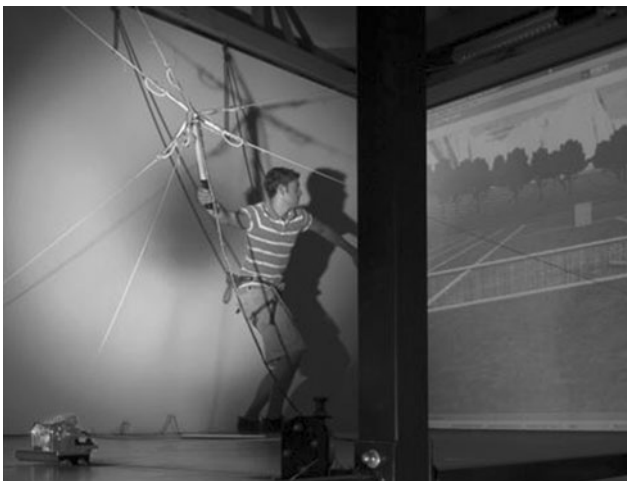
Fig. 1 The r^3 system: the reconfigurable, tendon-based robotic device developed at ETH, Zurich, for the tennis application (Marchal-Crespo et al. 2012)
