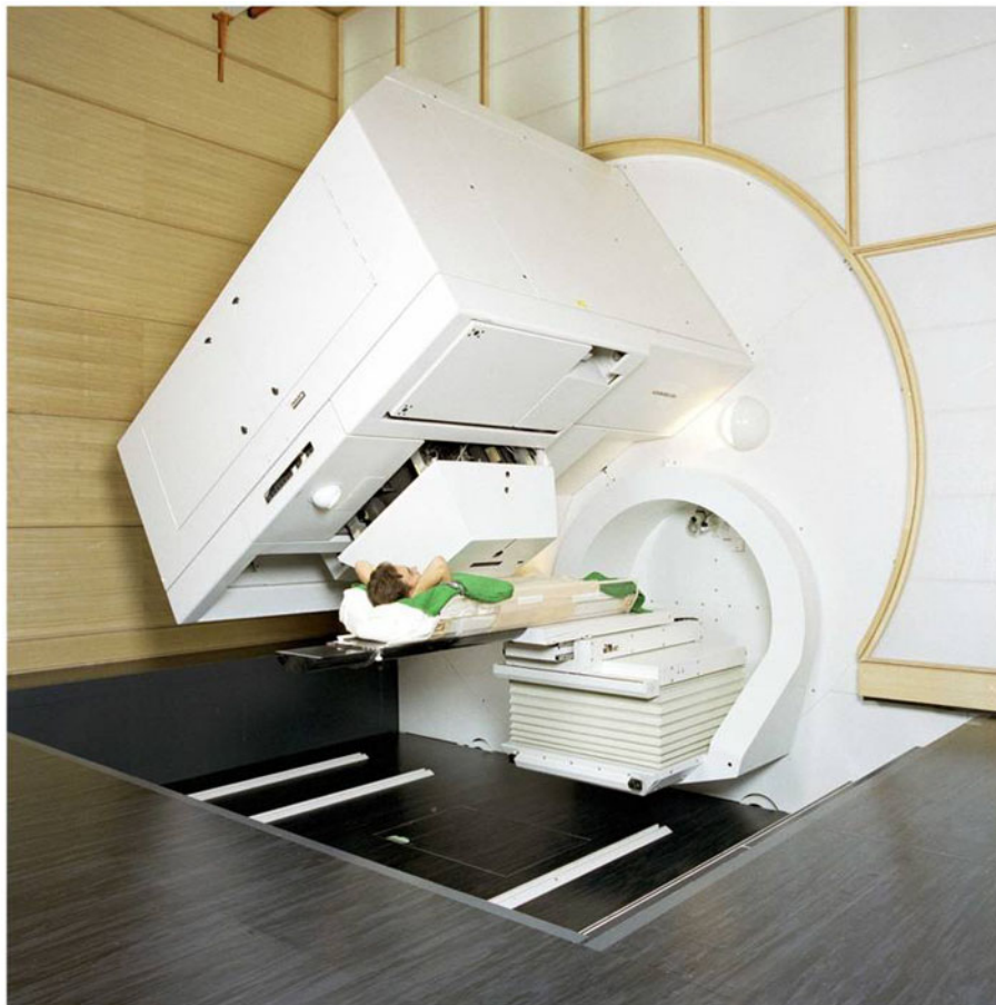
Fig. 1. Photograph of Gantry 1, the system used since 1996 for treating patients with pencil beam scanning at PSI.
