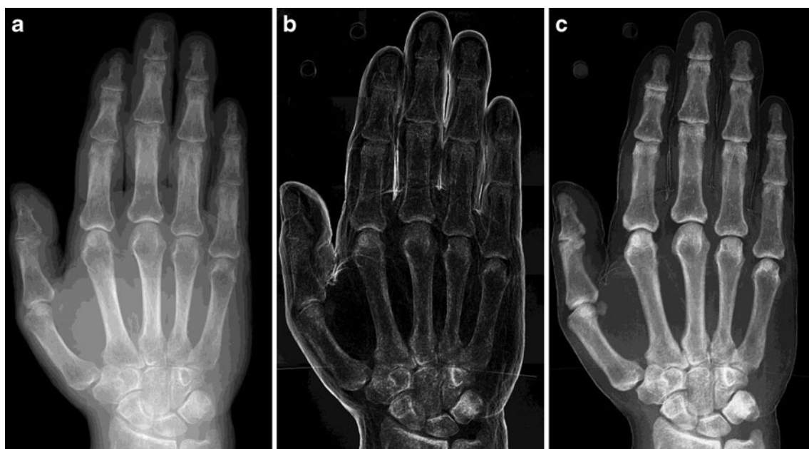
Fig. 2 Images of a human cadaver hand in the three contrast modes, acquired with the grating interferometer: a standard absorption contrast, b phase contrast (PC), and c dark-field contrast
