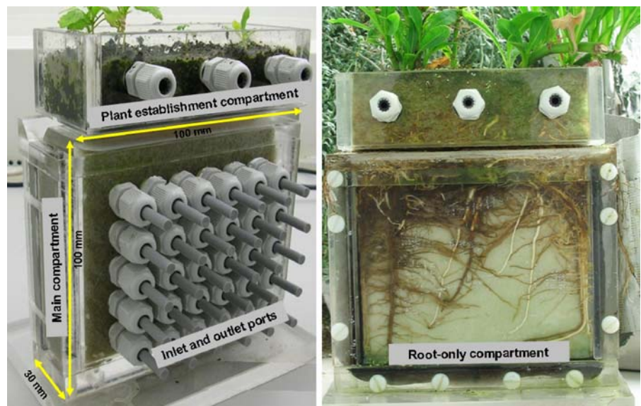
Fig. 1 The rhizobox set up with a view of the outlet and inlet ports (left) and the root-only compartment (right)
