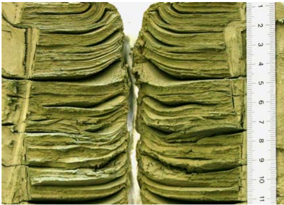
Fig. 1 Sample of Swiss lacustrine clay taken in Wauwil from a depth of 27 m, showing the typical varved texture of fine-grained lacustrine deposits (ruler unit in centimetres)
