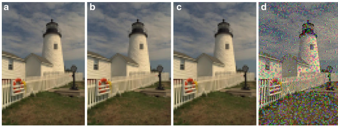
Figure 10 Proposed system with DCT at V_{dd1} and IDCT at a V_{dd_{nom}} , b V_{dd1} , c V_{dd2} , d Conventional System at scaled V_{dd1} .
