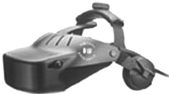
Fig. 2. Head-mounted display (HMD) used during this study (manufacturer: Virtual Research).
