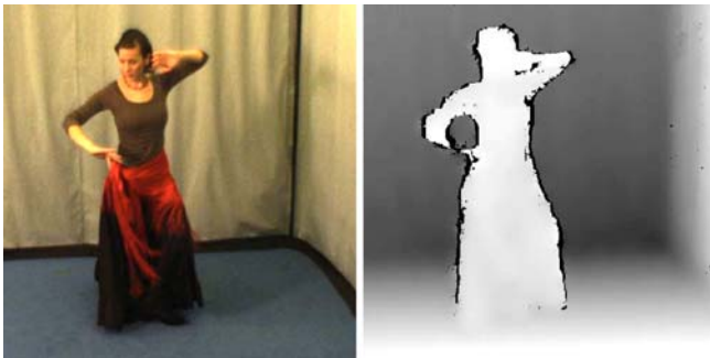
Fig. 9. Example of an acquired color image (left) with corresponding reconstructed depth map (right)
