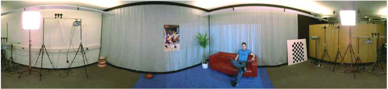
Fig. 8. Our 3D video studio consisting of four acquisition bricks. Structured light patterns illuminate the scene to support the 3D reconstruction
