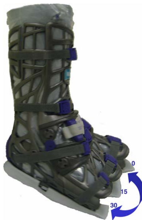
Fig. 1 The orthosis used from day 10 to the eighth week, permitting variable degrees of static or dynamic plantar flexion
