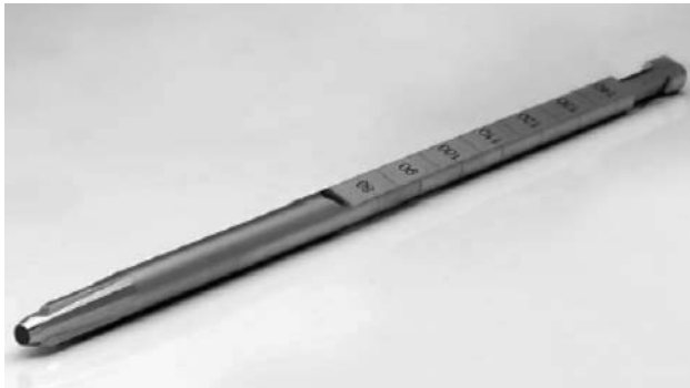
Fig. 3 The cannulated rod like mechanical probe: Central cannulation allows insertion over the guide wire. The tip consists of three blades placed at an angular distance at 120^\circ each. A measurement scale at the tail allows control of the insertion depth of the probe
