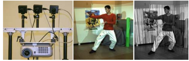
Fig. 2. 3D video brick with cameras and projector (left), simultaneously acquiring textures (middle), and structured light patterns (right)
