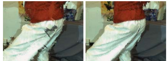
Fig. 7. Enforcing photo consistency during view merging: Without (left) and with (right) enforcement
