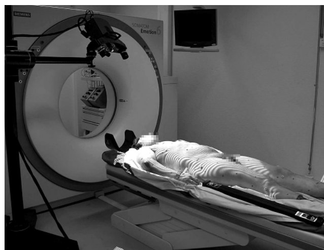
Fig. 1 ▶ 3D surface scanner ATOS III and 6-row multislice CT scanner, used by the Virtopsy group in Bern. Notice the wave pattern, projected onto the corpse by a projector unit and captured by two CCD cameras mounted beside the projector
