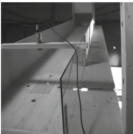
Fig. 1 Front view of the granular chute: force plate in the centre, ultrasonic flow height sensor above it and optical velocity sensors on the ground are visible. During the experiments the high-speed camera is installed in the void space behind the glass wall
