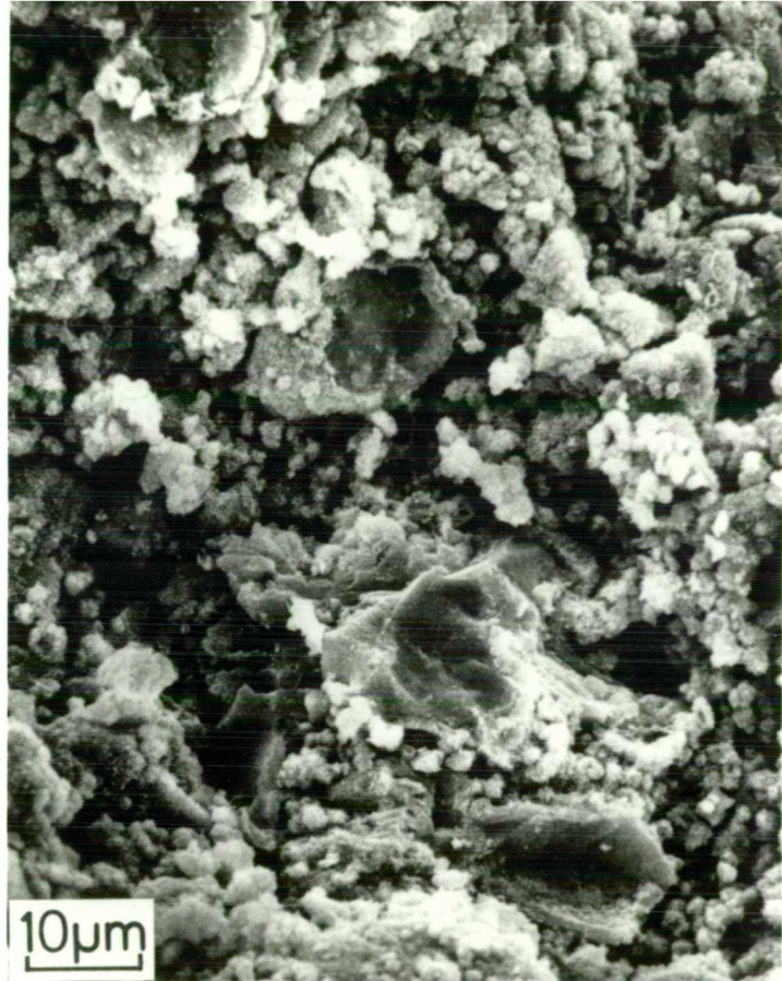
Plate 6.1 Fracture surface of 1 day old cement paste
