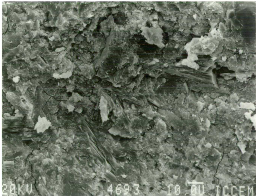
Plate 5.13 Fracture surface of cement hydrated for 69 days (D44)
