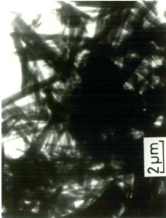
Plate 4D.3 Microstructure of C 4 AF(NBS) in the HVEM (a) 1 day (b) 4 days
