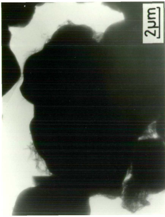
Plate 4B.4 Belite in the HVEM Hydrated for 8 days
