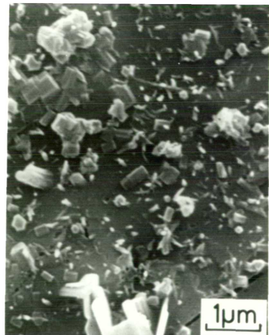
Plate 5.8 Dried fracture surface of 3 hours old cement (D44)
