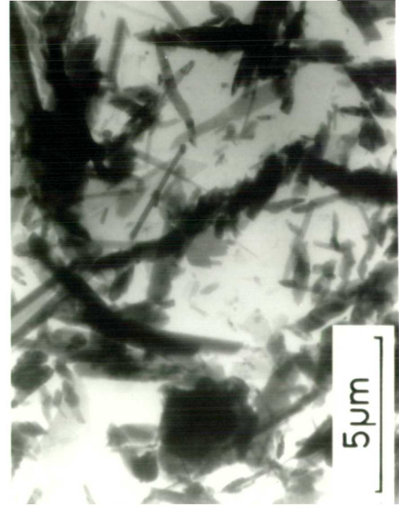
Plate 4D.2 Hydration of C 4 AF (NBS) with hemi- hydrate in the HVEM, (a) 10 minutes (b) 1 hour
