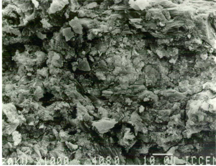
Plate 5.12 Fracture surface of cement hydrated for 1 week (D44)
