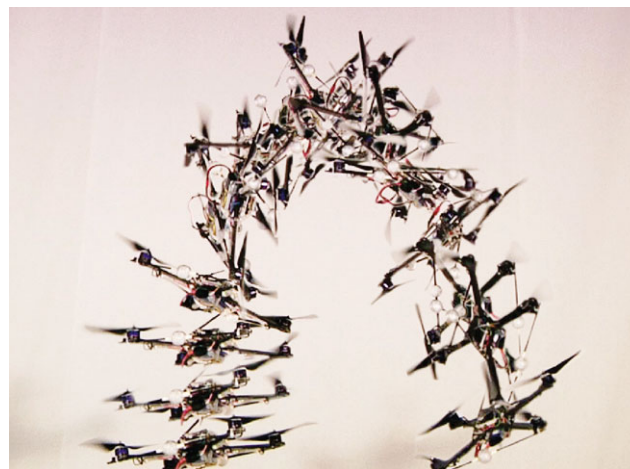
Fig. 1 Composite time-lapse photo of a quadrocopter performing a triple flip designed and learned using the described algorithm. The individual snapshots are offset horizontally for clarity—the vehicle returns to the original spot in the actual maneuver. The maximum commanded turn rate is 1800^\circ/\text{s} . The complete hover-to-hover maneuver takes 1.6 seconds
