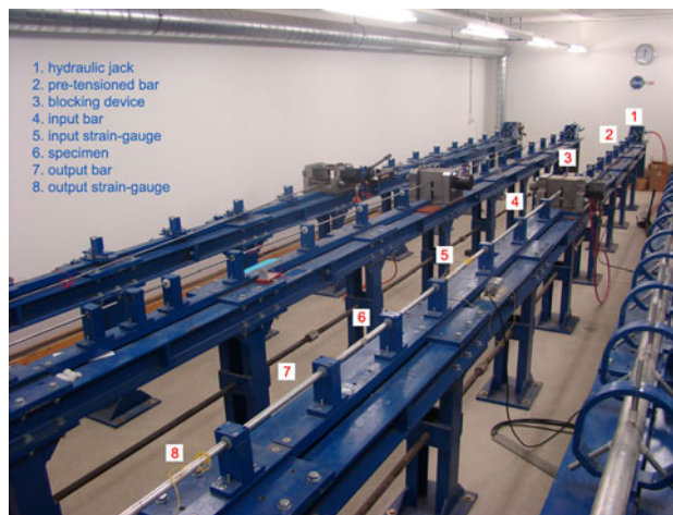
Fig. 2 DynaMat Laboratory: set-up for the high strain rate tensile tests on specimen \varnothing = 20 mm
