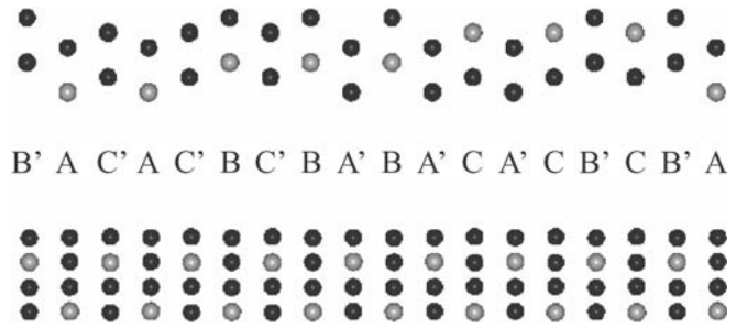
FIGURE 2 The projection of the unit cell of the martensitic \beta'_1 phase in two directions. The symbols A, B, ... denote the six types of close-packed stacking planes (data taken from [24])
