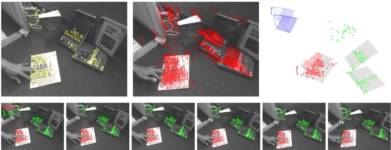
Fig. 9 Segmentation of the “magazine” sequence. Top : first frame with feature points superimposed, last frame with feature tracks superimposed, 3D view of reconstructed motion. The gray rectangles have
