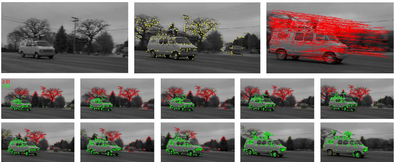
Fig. 10 Segmentation of the “delivery van” sequence. Top : first frame, fifth frame with feature points superimposed, last frame with feature tracks superimposed. Bottom : recovered segmentation through the se-
