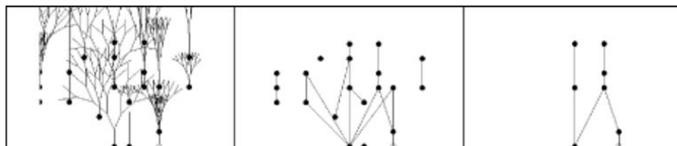
Fig. 6 Growth of axonal connections in the 2D brain space, pruning of axons that do not connect to other neurons, and pruning of all neurons that are not connected to input, output, or other parts of the network. From Nolfi et al. [57]
