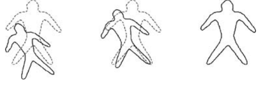
Figure 7. Minimization of F_{\text{shape}} with the flow given in Eq. (12), \phi and \mathbf{x}_{\text{pca}} being fixed. The row of images represents the affine registration of a prior shape in solid line into an active contour in dotted line.
