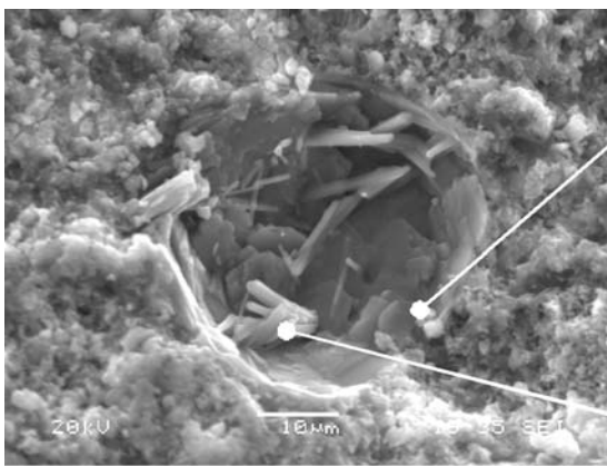
Fig. 5 SEM-EDS analysis of a pore recovered by portlandite (EDS spectrum a) and ettringite needles (EDS spectrum b)
