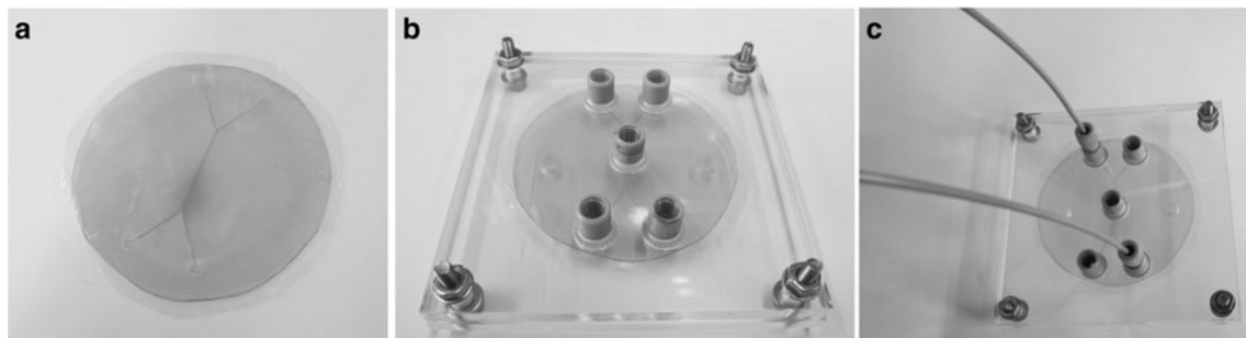
Fig. 1 Microfluidic device. The scheme (top) shows the setup of the microfluidic device. The 12 \mu\text{m} thin PEEK foil containing the 10 \mu\text{m} wide micropore is bonded to the 300 \mu\text{m} thick PEEK foil containing the microfluidic channel structure (a) and the bonded sheets
