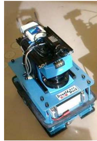
Fig. 6 The autonomous robot Donald Duck. Its controller consists of a VME standard backplane with a Motorola PowerPC 604 micro-processor clocked at 300 Mhz. Among its peripheral devices, the most important are the wheel encoders, a 360° laser range finder and a grey-level CCD camera (not used here)
