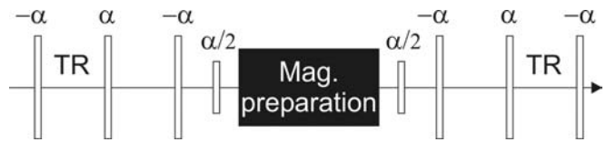
Fig. 11 Principle of contrast modification during the steady state of b-SSFP. The steady-state magnetization is stored in z-direction before magnetization preparation, and is recalled after preparation
