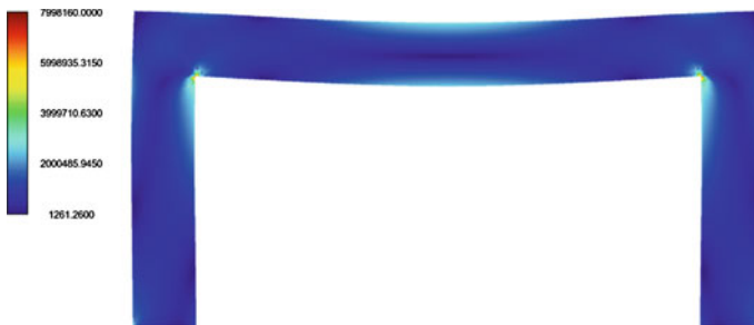
Fig. 14 Von Mises stresses (displacement is magnified for visualization purposes)
