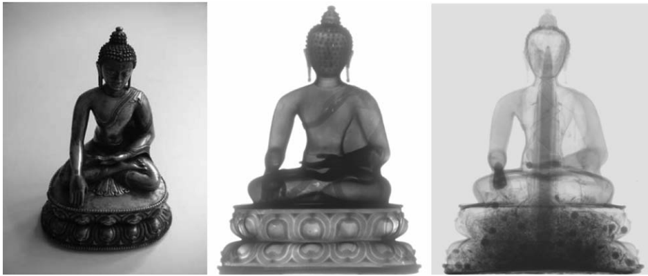
Figure 1. A sealed Buddha figure (left) (about 20 cm in height, photo) – Sakyamuni, Bhumisparsha Mudra, West-Tibet, 14th–15th century – was investigated with X-rays (150 kV tube voltage, middle) and thermal neutrons (right). Whereas the X-ray image only shows the outer metallic brass cover, neutrons can ‘see’ also the hidden organic cultic enclosures (wood, dried plants, cord) (courtesy Prof. M O Speidel, CH).
