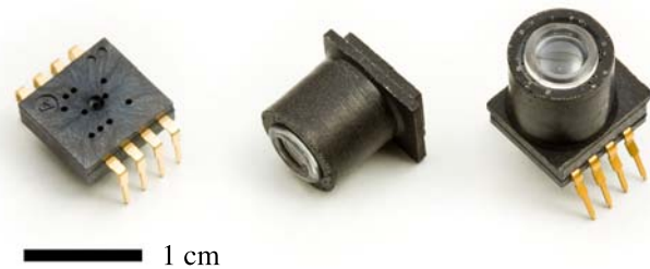
Fig. 10 From left to right: the Avago ADNS5050 optic mouse sensor, the custom-designed optics based on the Philips CAX100 collimator lens ( f = 10 mm) and the assembled optic flow detector (weighing 0.8 g)
