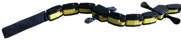
Fig. 8 The Salamandra robotica II amphibious robot
