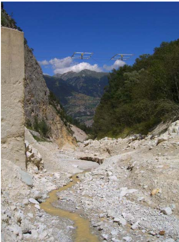
Fig. 5 The two radar sensors at check dam 10 (Fig. 2) that measure flow depth as part of the detection system (downstream view)
