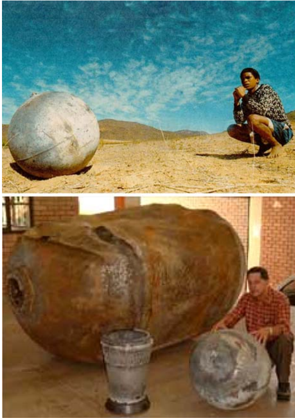
Fig. 6 Parts of a Delta II upper stage, which survived the atmospheric reentry
