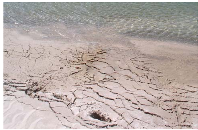
Fig. 2 Typical quicksand bed at the shore of a drying lagoon in Lençóis Maranhenses (Maranhão state, North-East of Brazil). Beyond a threshold pressure p_c , the crust of the quicksand breaks in a brittle way leaving a network cracks, and the material collapses. The maximum penetration depth for the human body was not greater than 1 m
