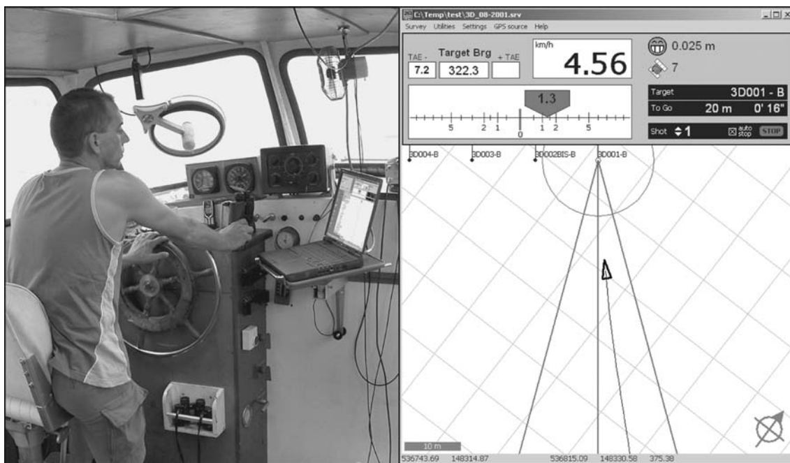
Figure 4. Setup of laptop with navigation software and screen display of the specially developed program (GPS_shot). This example shows navigation monitoring while the ship sails to the profile starting point. Top of window shows a number of navigation parameters including current target bearing, ship speed, lateral deviation from target line (large arrow), number of GPS satellites used and accuracy with which coordinates are determined.
