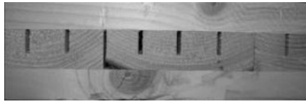
Fig. 11 Cross-section view of the strip taken from panel R_0.08_3L_A_P1: Knots, pitch pockets, deviated grain and grooves affect nearly the whole respective layers
