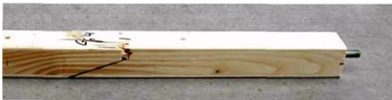
Fig. 7 Tensile failure in timber
