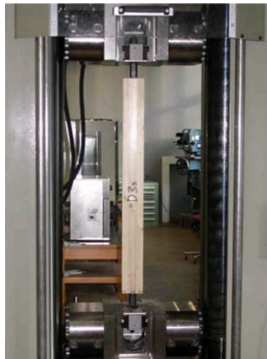
Fig. 5 Tensile test of specimens in pull-pull configuration
