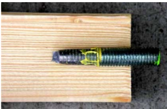
Fig. 3 Steel failure (yielding of the rod)
